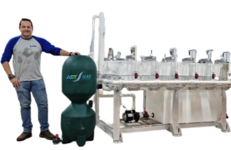
The INCUBRAS supports a dozen 6.9-liter McDonnel Jars in a closed recirculating format with a total system volume of 220 gallons.
